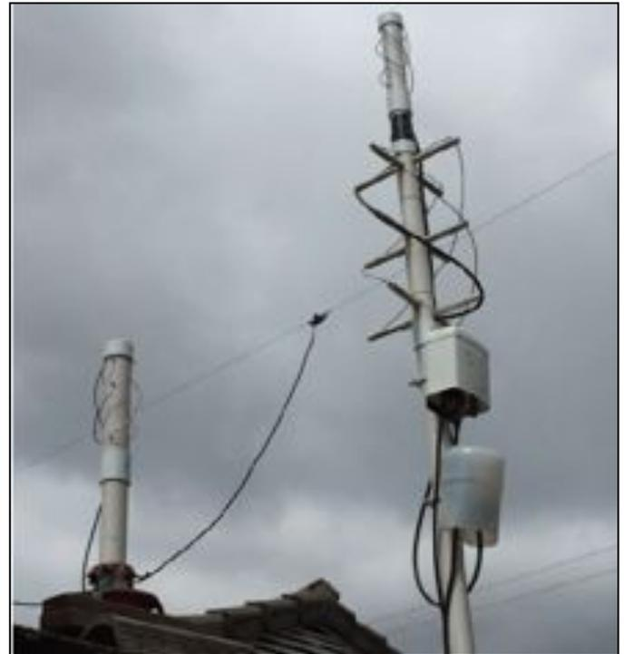
**Figure 3: AA6QI's QHA's (left - 70cm LHCP; upper right 70cm RHCP; lower right 2m RHCP). Note that there is a 40m dipole in the background that is not part of the QHAs. The plastic covers below the antennas house diplexers and preamps for each band.**
