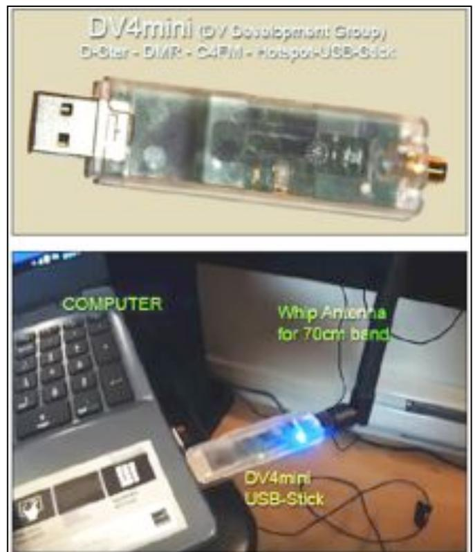
Figure 10: DV4mini VHF/UHF multi-mode dongle
