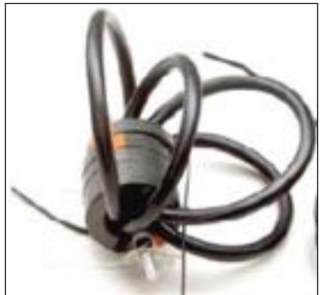
**Figure 2: A choke consisting of 5-turns through five 2.4" O.D. mix 31 ferrite cores from Jim Brown's paper.**
