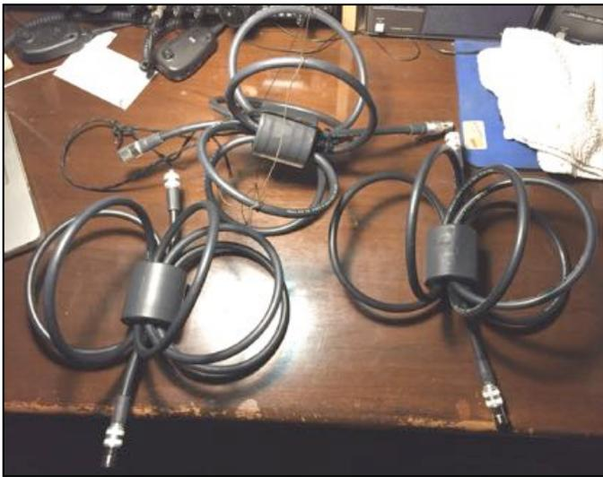
**Figure 5: Three common-mode chokes aimed at reducing 80m & 40m noise levels in B310 and B329.**
