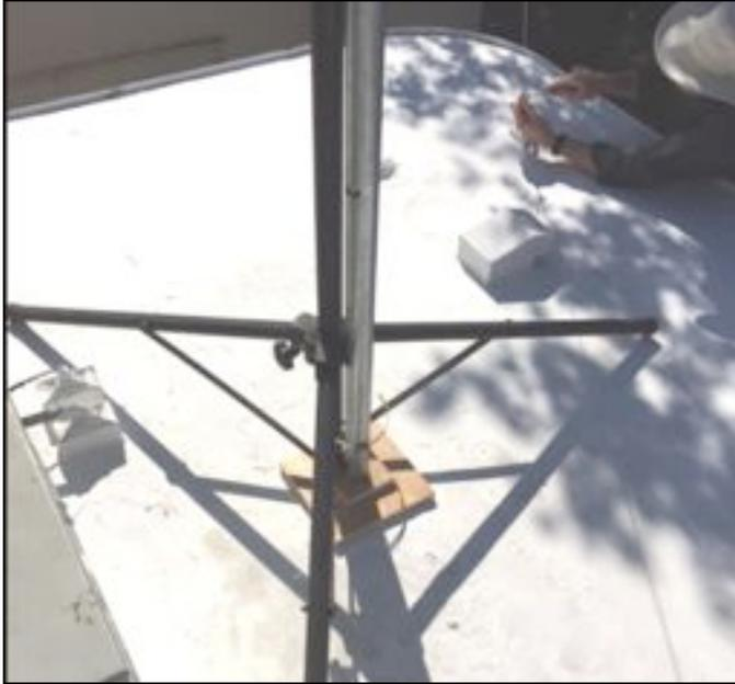
**Figure 2: R7k antenna tripod base on the roof of B329 (upper right- Bill Weber tightening a guy wire)**
