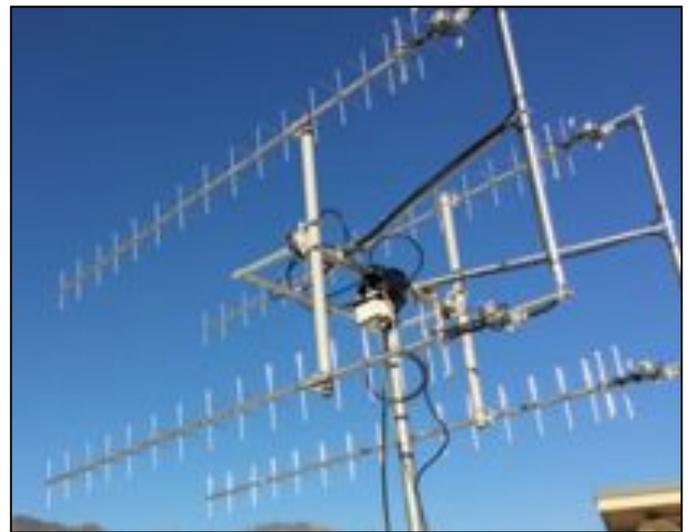
Figure 6: JPL CubeSat UHF tracking antenna system
