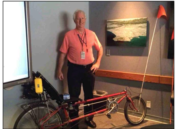
**Figure 2: Courtney Duncan N5BF with his APRS-equipped 1991 Ryan Recumbent bicycle. His Byonics Micro-Trak APRS transmitter is in the yellow case.**
